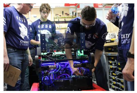
Step four of the design process is to make something called a "prototype." A prototype is the first working design of the machine. The finished machine usually looks different then the prototype, but the prototype includes the most important parts of the design so engineers can test how they work! After engineers create a prototype, the fifth step of the design
